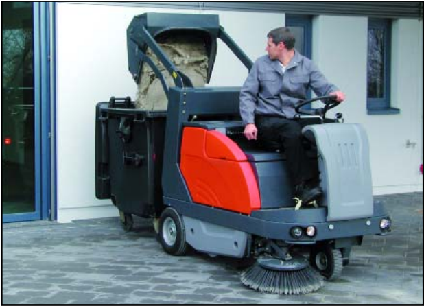
The high dump hopper can be easily emptied into large containers.
