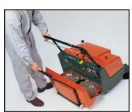
**Easy to empty hopper:** The large capacity hopper recovers a large variety of debris and can be filled to 100% capacity due to the overthrow sweeping method. It can be easily emptied using the two ergonomic handy hopper inserts.
